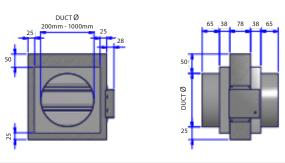
FOR DUCT WIDTHS 200MM - 1000MM WITH HEIGHTS OF 100-199MM
