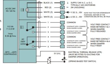
DIAGRAMS SHOWS ACTUATOR IN FULLY CLOSED STATE
