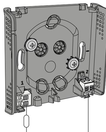
24V AC/DC Digital input for external connection.
