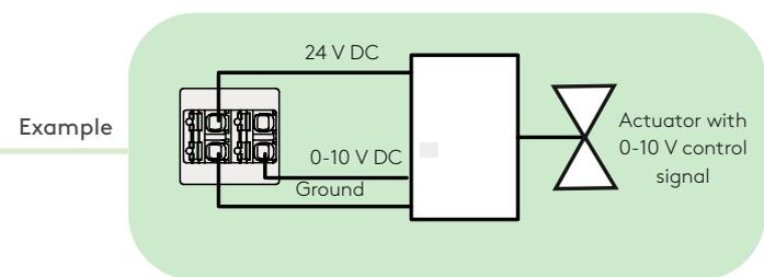
Connection of actuator with 0-10 V control signal.
