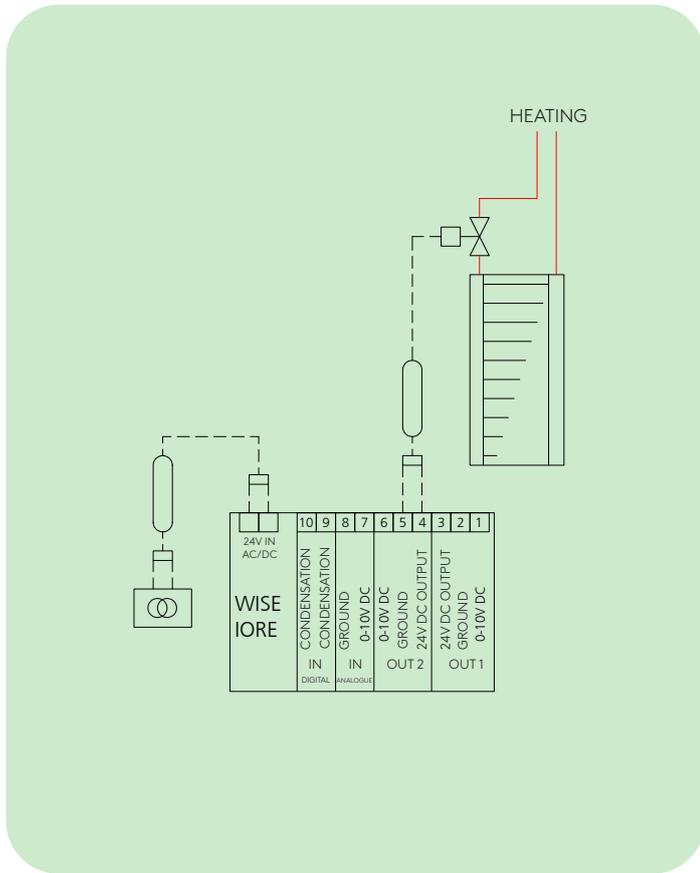
IORE controlling radiator heating (24 VDC PWM, thermo-actuator)
