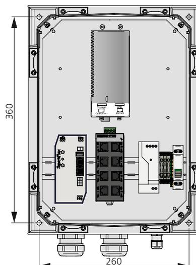
Holes for installation (mm), SuperWISE II 2K, SuperWISE II 2K SC. 4x installation screws (clearance hole  $\varnothing = 8$  mm), screw selection based on the substrate.
