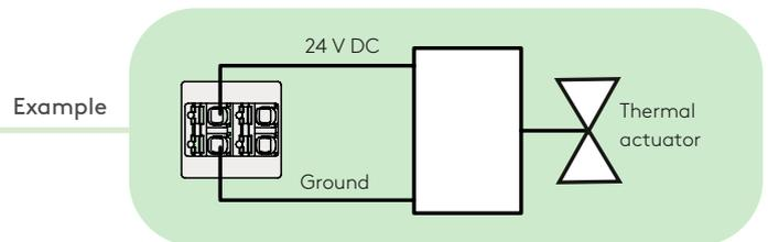
Connection of thermal actuator
