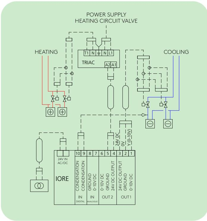
IORE controlling heating (24VDC PWM, 2 or more thermo-actuators) and cooling (24 VDC & control 0-10V, 2 or more actuators) as well as condensation sensor (TRIAC)
