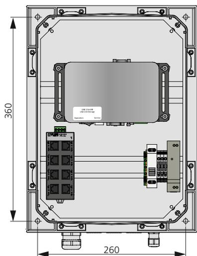
Holes for installation (mm), SuperWISE II, SuperWISE II SC. 4x installation screws (clearance hole  $\varnothing = 8$  mm), screw selection based on the substrate.
