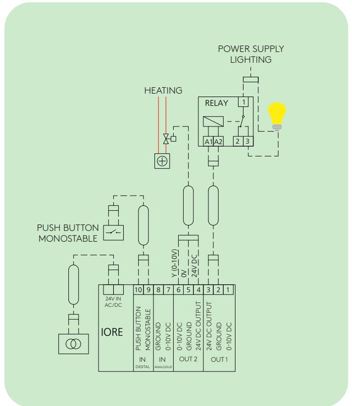
IORE controlling lighting and heating, as well as push button for lighting
