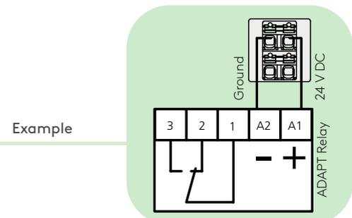
Connection of relay for connection of 3 or more actuators
