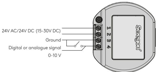
1. Connection of the power supply G0 0V AC/-0V DC
