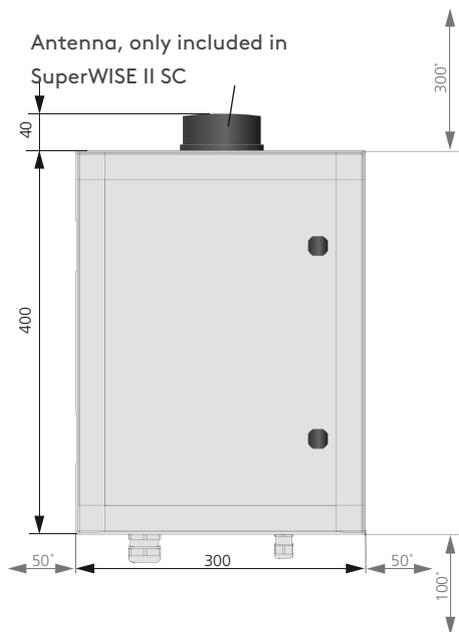
SuperWISE II, SuperWISE II SC, measurement figure (mm).
