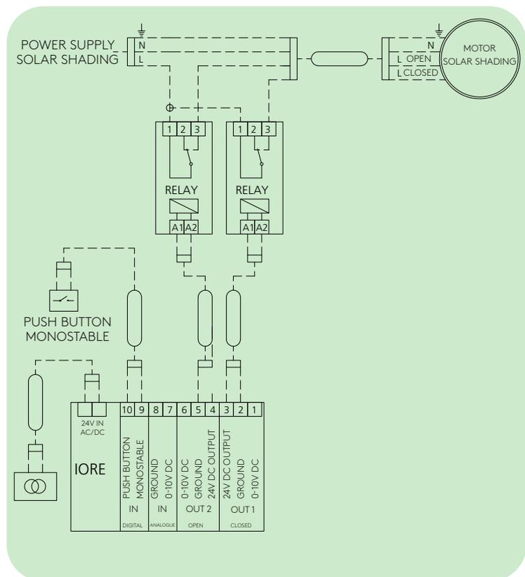
IORE controlling solar shading and push button for manual control of solar shading
