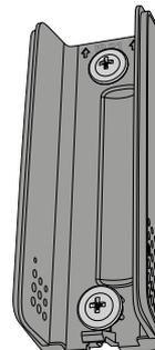
1. Screw mounting on the wall, screw max. Ø4.5 mm, min. length 20 mm, screws not supplied.
