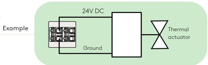
Connection of thermal actuator
