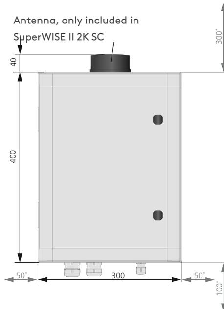
SuperWISE II 2K, SuperWISE II 2K SC, measurement figure (mm).
