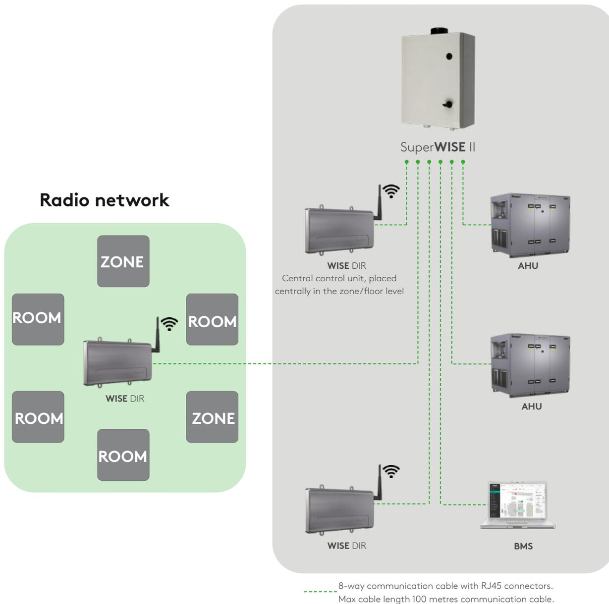
**NOTE!** The radio and operating networks shown in this document are only examples of how these can be structured. The radio and operating networks are built up depending on the need and function in the building project.
