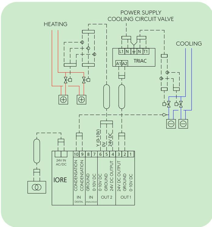
IORE controlling heating (24 VDC & control 0-10V, 2 actuators) and cooling (24 VDC PWM, 2 thermo-actuators) as well as condensation sensor (TRIAC)
