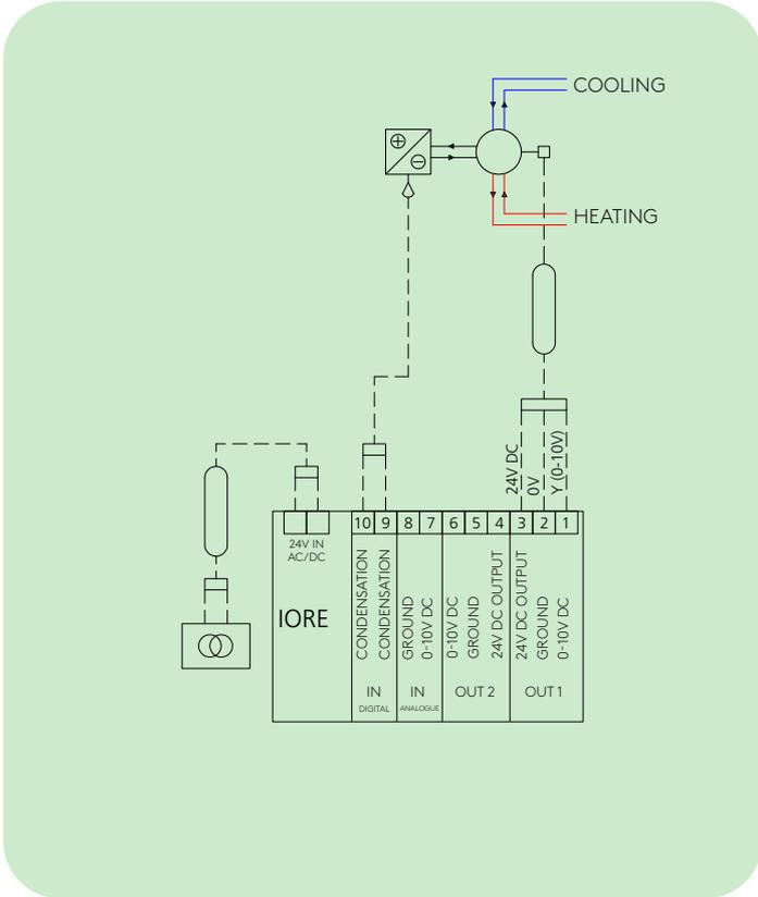
IORE controlling 6-way valve/CCO valve (24 VDC & control 0-10V)
