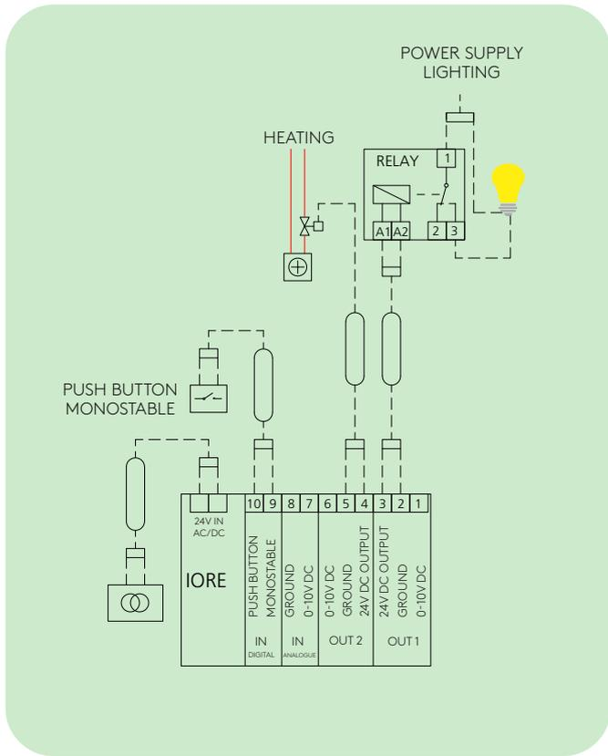
IORE controlling lighting and heating, as well as push button for lighting
