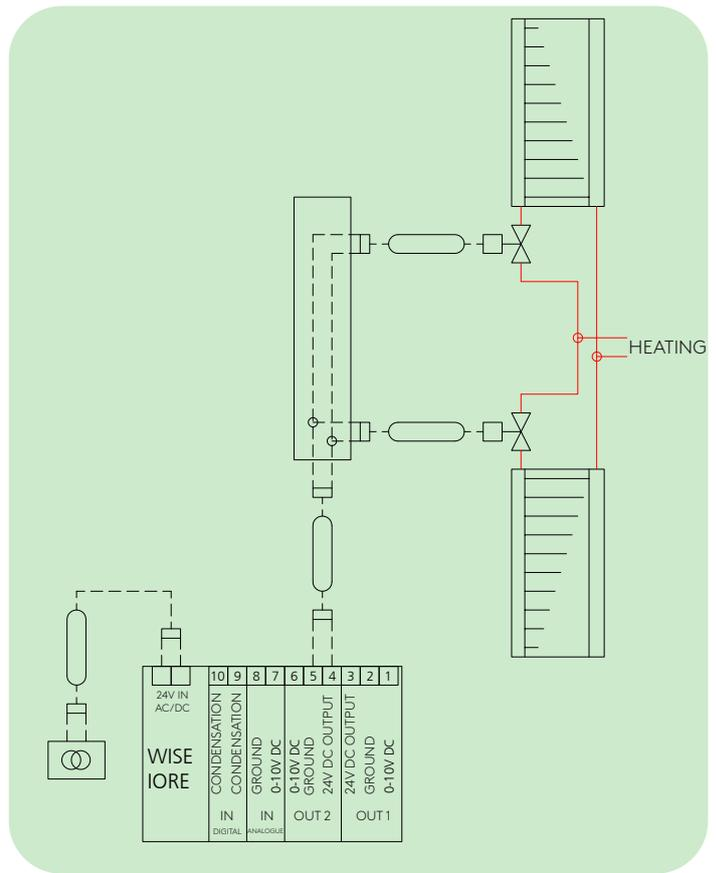
IORE controlling heating (24 VDC PWM, 2 thermo-actuators)
