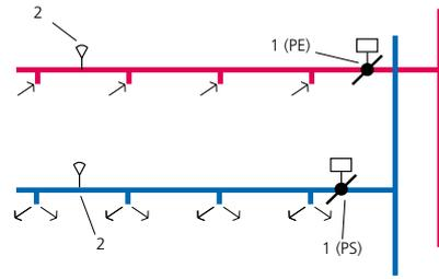
Constant pressure regulation, recommended installation 2/3 out in duct, max 100 m, 1: WISE Damper, 2: WISE DPS
