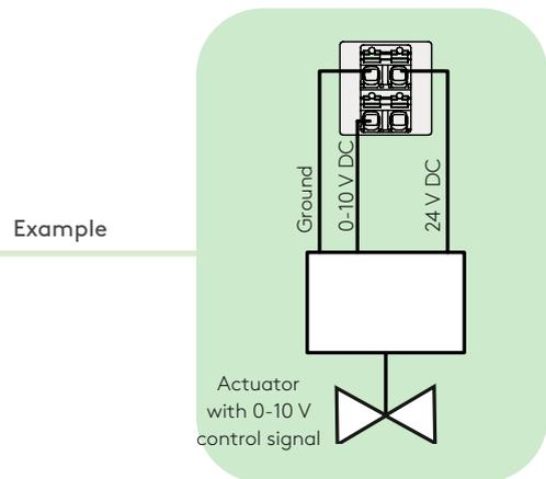
Connection of actuator with 0-10 V control signal
