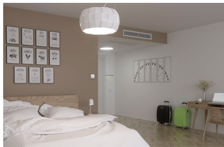
Hotel room with setpoint selector switch, waterborne cooling and heating as well as demand-controlled air regulation. Key card holder for occupancy.
