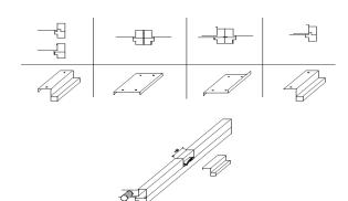
For large pieces of equipment, the square tubing should be additionally secured with connecting clamps
