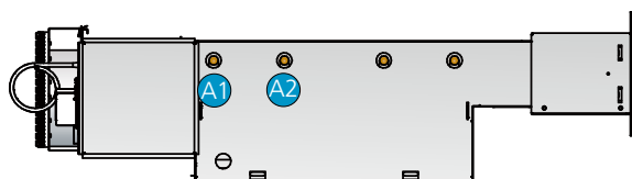
Figure 22. Water connection on the right-hand side (R). A1 = Cooling water, supply B1 = Heating water, supply A2 = Cooling water, return B2 = Heating water, return
