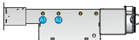
Figure 24. Water connection on the left-hand side (L). A1 = Cooling water, supply B1 = Heating water, supply A2 = Cooling water, return B2 = Heating water, return
