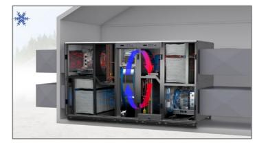
When the need for supplemental heating increases, the GOLD RX/HC starts the integrated heat pump. The heat pump components are built into the unit, which boosts operating efficiency further. The heat pump coils take up heating energy not recovered by the rotary heat exchanger. The GOLD RX/HC also has an exceptionally wide working range, and continues to generate heating even at an outdoor temperature as low as -25°C.
