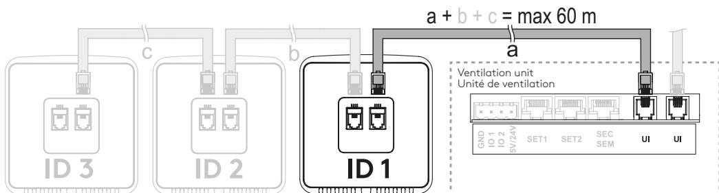
**EN** The total length of the control cables must not exceed 60 meters. Use ready-made 20 m cables. Never cut/extend the cables. Connect only one panel to a Wi-Fi network. The control panel is not suitable for installation in a multi-switch frame.
